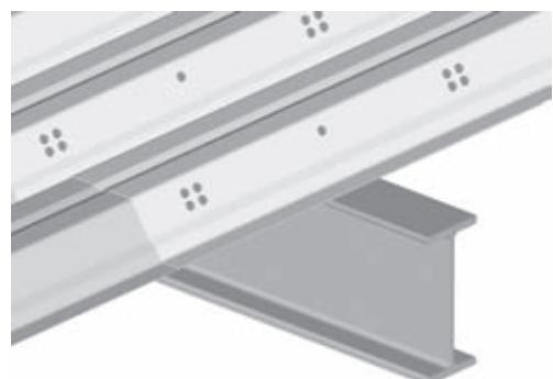
Self-drilling screws should be used to join sheets together and fasten them to the construction support or steel frame structure.
